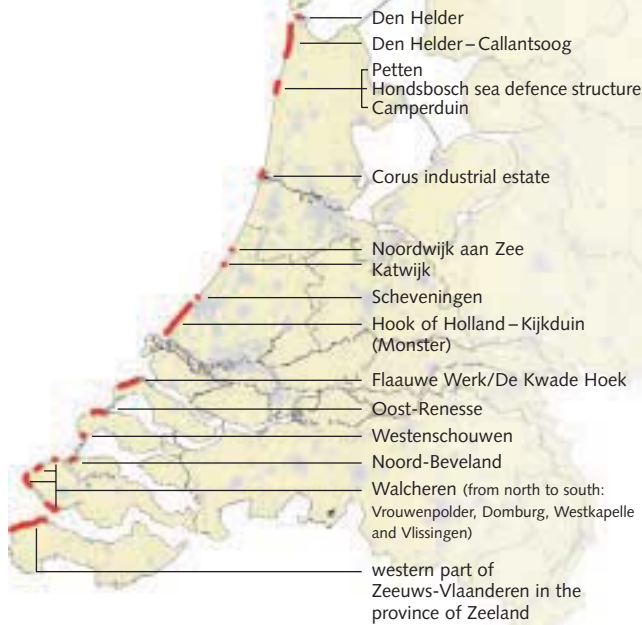
Weak links: areas in the Dutch coastal defences that need to be reinforced within the next 200 years
